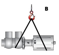
DN80 and DN100 Weight between 25 kg and 50 kg
