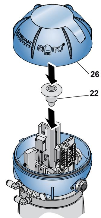
4 When the valve is in the close position set the proximity switch to have its lower quarter active sensing zone in correspondence with the upper part of the cam.
