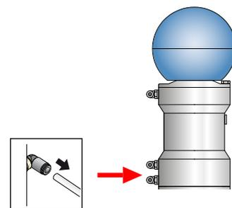
13 Remove the split annular ring spacer.
