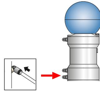
9 Adjust and regulate the proximity switch position until the lower middle section of the sensitive area is in correspondence with the upper edge of the upper shutter.
