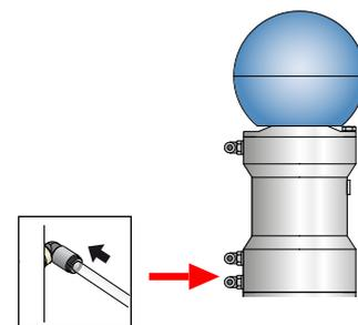
16     Seat lift upper shutter will open, with a stroke of 2mm
