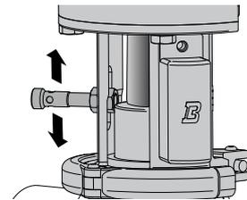
10 Fix the proximity switch in position with the external nut.
