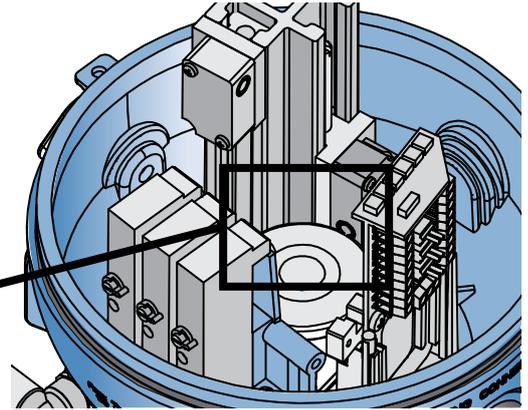
5 Activate the lower lift with regulated air at 6 bar in the upper air connection in the actuator.
