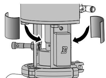
8 Activate the upper seat lift with regulated air at 6 bar in the lower air connection in the actuator.
