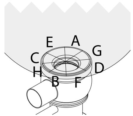
Assemble the valve after welding.
