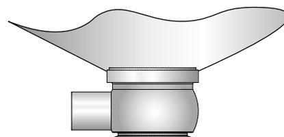
Only use pulsed arc welding and remember no gap between flange and tank plate.
