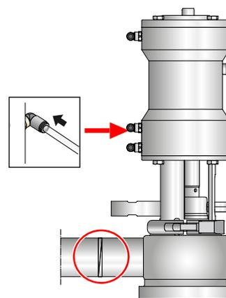
Weld it care/ try to make a stressless welding to avoid deformation on sealing areas. Check the valve for regular operation after welding
