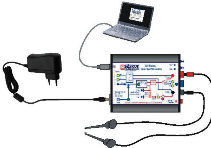
Connect the modem to the Flushing unit, pin7 and pin10, with the use of “alligator hooks” The polarity does not matter. Only make sure there is a load of 250ohm between them, otherwise the HART communication will not work. If the load resistor has been removed from the flushing unit during initial startup, connect to the corresponding load resistor within the automation system.
