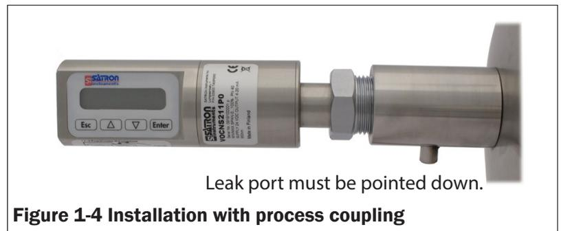
Leak port must be pointed down.
