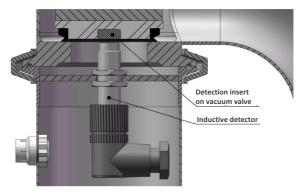
If the valve is fitted with a vacuum part spring operated, rod (Ref.5.7) is muni of 2 nuts (Ref.5.9) in its bout which allows an inductive detector.
