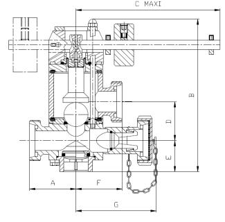
Connect the collection chamber (can be rotated 360°) on a duct with no back pressure. When attaching the bunging valve system, do not force any of the connections.
