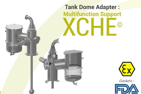
The XCHE is a device placed on the dome of a tank. At a single point, it can be fitted with equipment for pressure (SHP safety valve) and vacuum protection (BOG or HSV-A vacuum break valves depending on diameters), for washing the tank, the XCHE and all its components, and for pressurising and recovering fermentation gases (CHE washing check valve). The XCHE is also equipped with additional taps, for stainless steel rupture disc and/or for pressure sensor.
